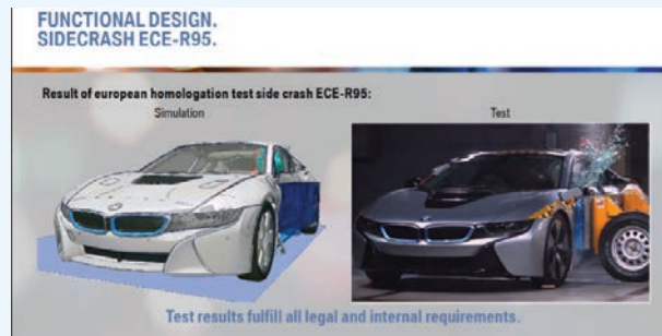
Figure 5: Validation of simulation models of side test crash simulation of the i8
